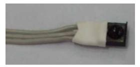
Adopt oblate three-way, wire and connect an infrared receiver to receive an external infrared.
